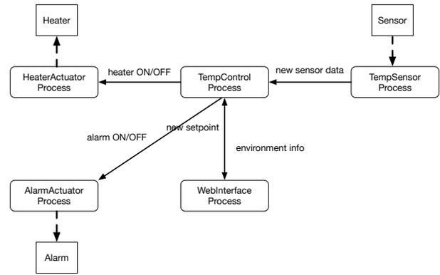
Fig. 2: Logic Illustration of Temperature Control Scenario
