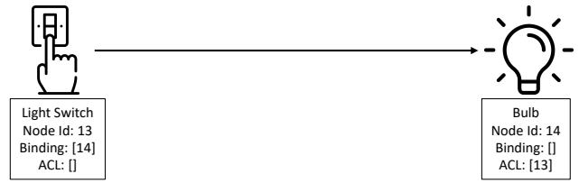
Fig. 4. Access Control and Binding List
